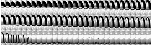
FIG. 4. Sequence of images for the cavity evolution. The tube is rotating at \omega=20 Hz while the vertical excitation is at 16.55 Hz. The equivalent time delay between photographs is 315 \mu\text{s} . Individual image height is 15.5 mm. The complete sequence shows almost one half of the excitation period.
